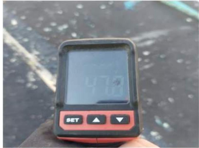
2. Substrate Temperature Reading
